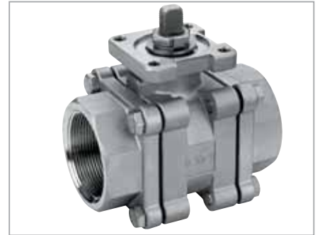
Above: The compact three-piece valve body design allows for disassembly and maintenance without removing the valve from the line.*
